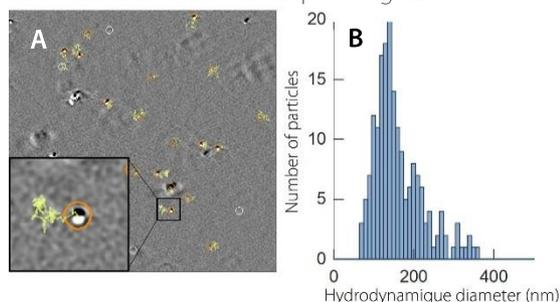
**Figure 1.** Purified lentiviral vectors images obtained with ILM **A.** Nanometric image where interference patterns of lentivirus can be detected and tracked to compute concentration and hydrodynamic diameter. **B.** Lentivirus size distribution histogram from tracked particles.
