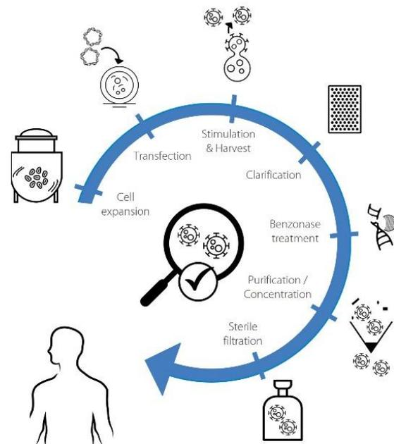
**Figure 2.** Lentiviral bioproduction process – upstream & downstream process
