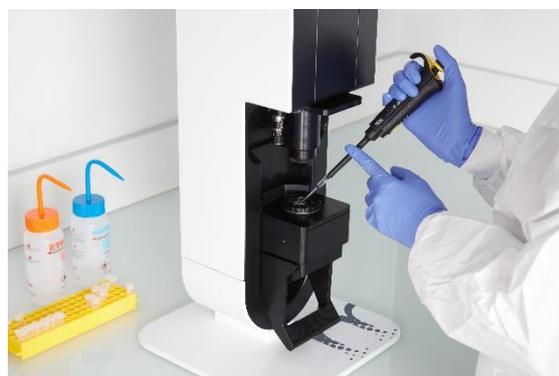
The microscope magnification and camera speed allow to perform analysis of small sample volumes (down to 5  $\mu$ L) in less than one minute.
