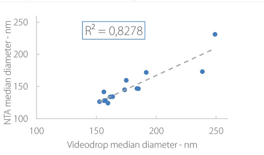
**Figure 6.** Median diameter measurement comparison between NTA and Videodrop on complex stress samples
