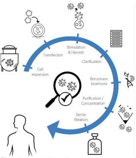
**Figure 2.** Lentiviral bioproduction process – upstream & downstream process
